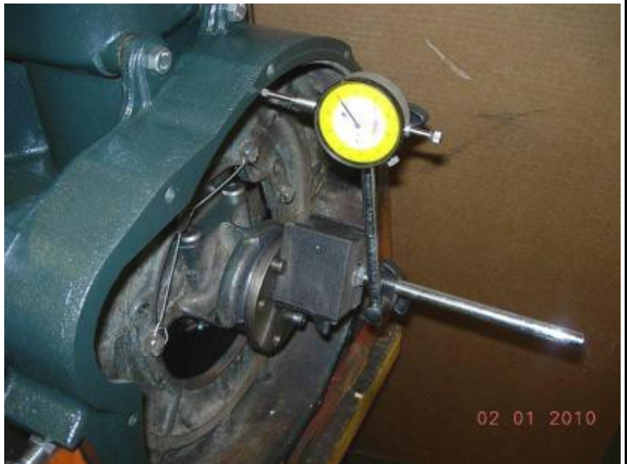
Dial indicator and magnetic base installed on a Model A crankshaft
